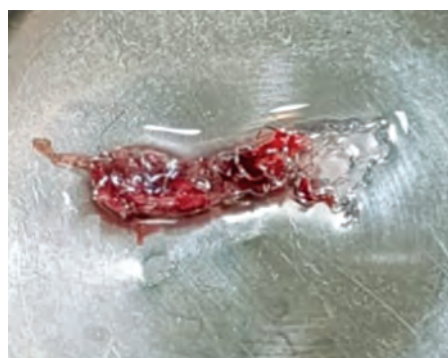
Fig. 4: Image of the retrieved deformed stent
